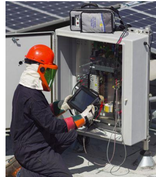
A worker using Solmetric PV Analyser for PV string testing
