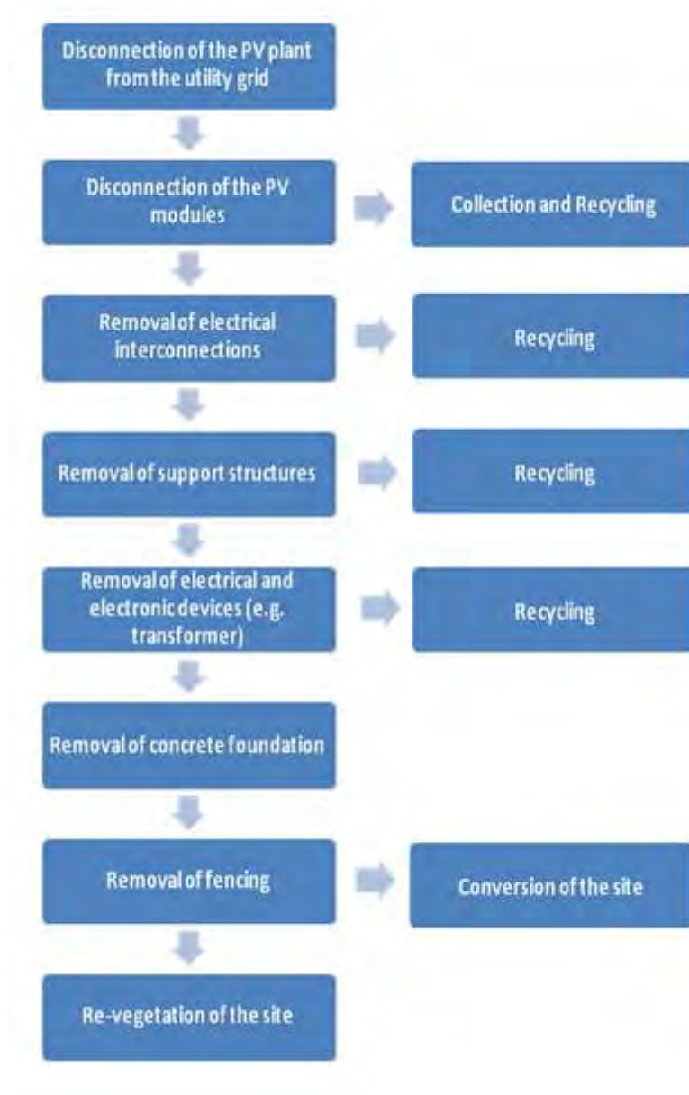
Figure II-48: Typical dismantling process
